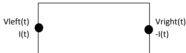
Figure 8.1. How variables map to physical ports in a resistor
