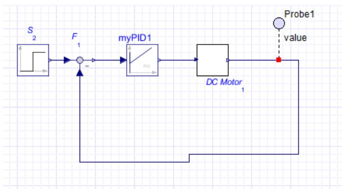
14. Click the probe button (probe icon) in the toolbar and then click the connection line between the **DC Motor** and **Feedback** component.
