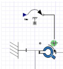
18. Click the input port of the **Torque** component and drag your pointer to the subsystem boundary.
