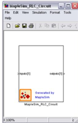
Double-clicking the block opens the mask that contains the symbolic parameters from the original model. This block can now be connected with any compatible Simulink blocks.
