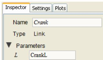
The **Crank** subsystem now inherits the numeric value of **CrankL** that you defined.
