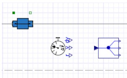
7. To connect the **Absolute Translation** component to the model, click the frame\_b connector. The frame is highlighted in green when you hover your pointer over it.
