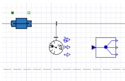
9. In the same way, connect the **r** output port ( *TMOutputP* ) of the **Absolute Translation** component to the demultiplexer Real input signal (u) port. This is the displacement signal from the sensor in x, y, and z coordinates. Since the slider only moves along the x axis, the first coordinate needs to be an output signal.
