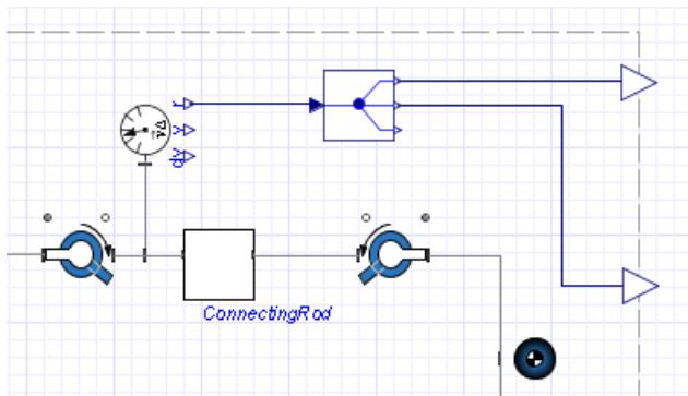
Since the crank is moving in the x, y plane, only the first two signals need to be outputs.
